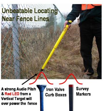
Hold the locator at an angle to the Fence the Mode Tone and Green LED will then appear. Next move the locator along the fence line. When a Strong Audio tone pitch & Red LED appears this will indicate a possible vertical target.
